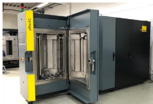
Figure 1. Industrial magnetron sputtering equipment at AIN.
